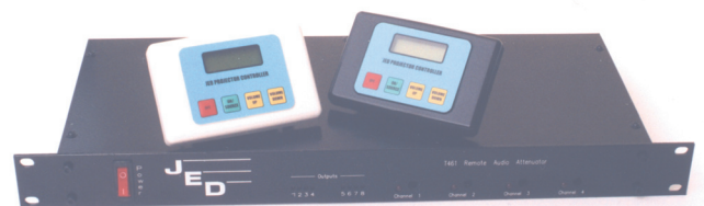
T461 audio switcher and attenuator, with T460s
