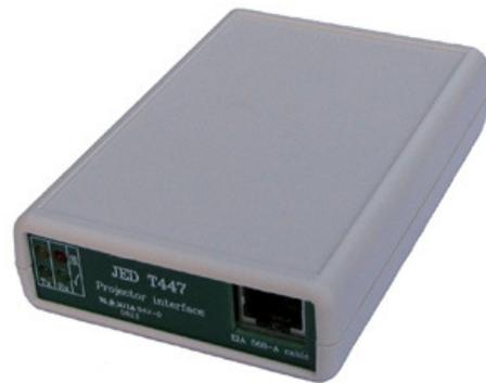
On one end of the T447 is a CAT5 connector to a CAT5 pre-terminated cable which is the only wiring to the T440 down on the operator’s wall or desk. ALL wiring needed passes through this CAT5 cable. On the left is a signal display showing transmit and receive data paths, green LEDs showing the RS232 negative rest state, and flashing red and yellow LEDs for the two transmissions, to the projector and the projector reply.
