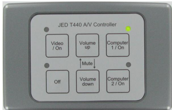
make sure the system is synchronised to the controller. At this point, the RED LED associated with the OFF key flashes once, if a proper “Off status OK” is received, and three times if it is not. (Some projectors don’t respond in the “Off” state so for these, the OFF LED just goes on.) The RED LED then stays ON to show the user the status of the whole system. This is a valuable test for users and installers, as it is so easy to test communications, with just one button press;
